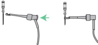
Clip the file clip to the metal shaft the file. Press in direction of arrow and clip file, then release to finish installation
