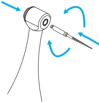
Hold down the push button on the contra angle and insert the file. Turn it back and forth until it is installed, and then release the button to lock the file into the contra angle.
