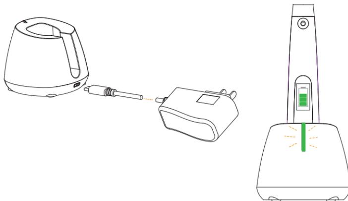
Connect the USB cable to the unit power connector, and plug the other end into a power outlet.
