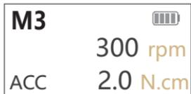
The motor rotates forward rotation (clockwise rotation), when the TORQUE is at about 70% of the setting torque for a long time, it will automatically reverse and resume forward rotation after the resistance disappears.
