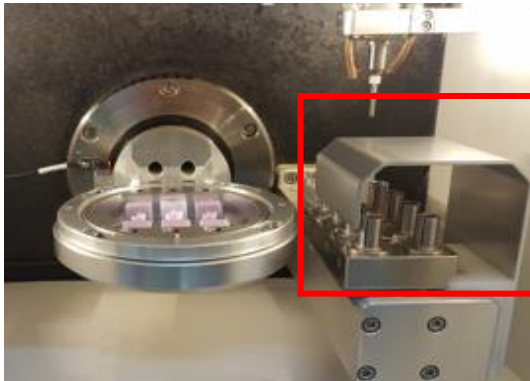
<DS200- 4W/4WA > ATC cover for 4 axis and wet milling
