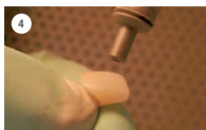
4 Perform Almina sandblast on the surface of the unpolished area of the crown (50~70µm, 30psi)
