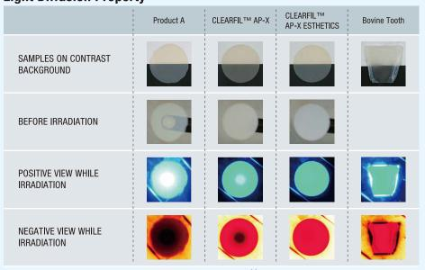
Composite Resin discs appearance while being irradiated by an LED light activation unit positioned 4.5mm below the disc. The outline of the light guide tip is easily observed for the light transmitting product but the CR disc shows a uniform appearance for CLEARFIL<sup>TM</sup> AP-X Esthetics (Source: Kuraray Noritake Dental Inc.).
