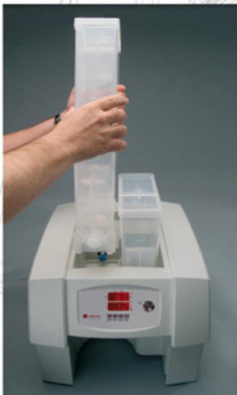
1) The access to the tank is immediate, and you can dismount it in a few seconds. You can load the tank from any comfortable position, without having to lift heavy bags over the machine. Besides, it prevents the powder generated during the operation to settle on the machine. Another advantage is the easy cleaning of the dosage system.
