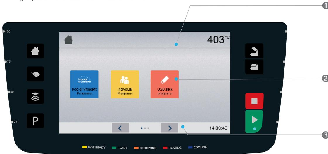
The user interface in the display is divided into three sections:
