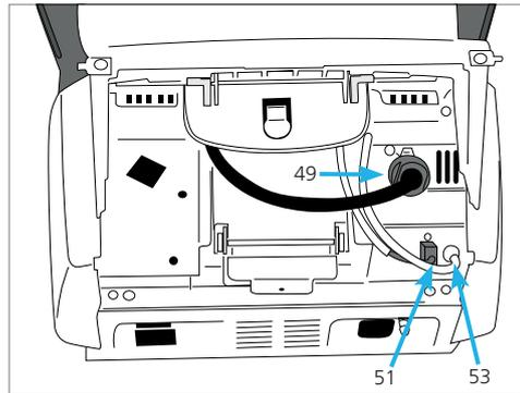
1. Insert the heater plug in the intended socket.
