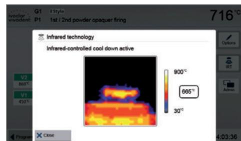
Once the object has reached the ideal removal temperature, the display shows a corresponding notification and the cooling time elapsed.
