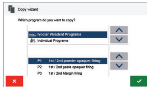
4. Select a target. Confirm the selection with the green button or close the copy wizard with the red button.
