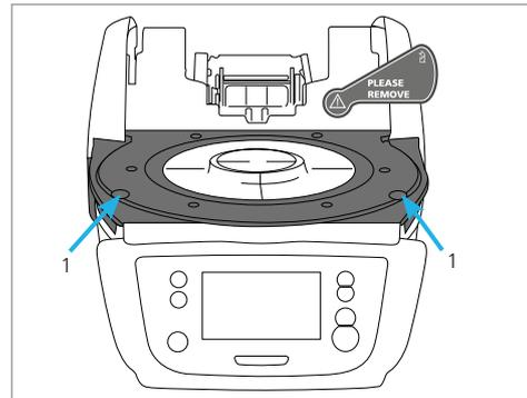
Place the cooling tray (2) on the frame plate (24). Make sure that the cooling tray is correctly positioned on the frame plate.
