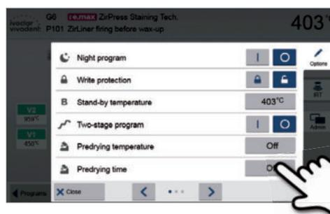
3. Enter the desired predrying temperature and confirm with the green button.
