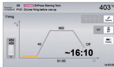
The IRT key (see Chapter 5.1.2) is used to switch to the view of the infrared camera during the closing and predrying process. The corresponding key is pressed again to return to the firing curve display.
