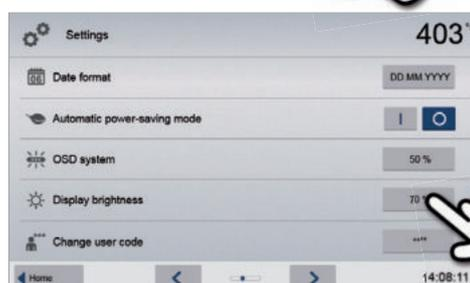
**4. Select the desired display brightness** in percent and confirm the entry with the green button or cancel the entry with the red button.
