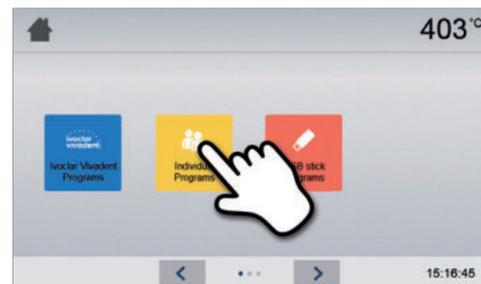
The next page of the home screen can be accessed with the **[Arrow]** button, where additional functions are available. The circles between the arrows indicate the number of pages. The current page is marked with a light dot.
