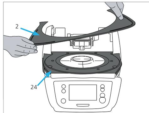
Secure the cooling tray (2) with the two screws (1).
