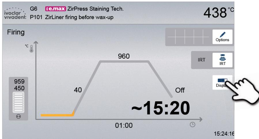
If the **[Display]** button is pressed while the firing curve is displayed, the remaining time will be shown. The remaining time indicator informs the user about the time that is left until the process is completed even from a distance. The remaining time is displayed in the center of the screen in large characters.
