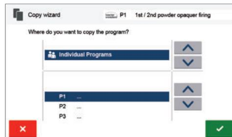
5. The copy process can be continued with the green button. The red button is used to abort the copy process.
