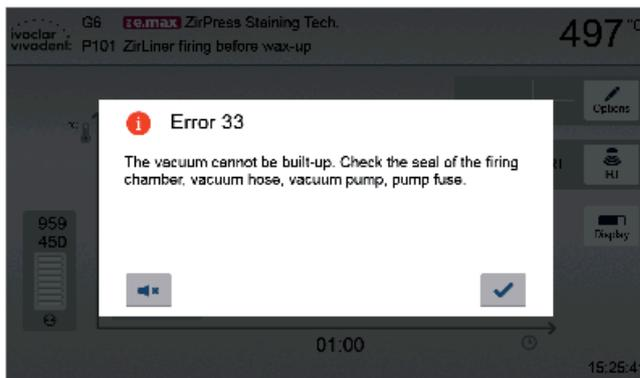
The acoustic signal and the error message can be acknowledged with the corresponding buttons.
