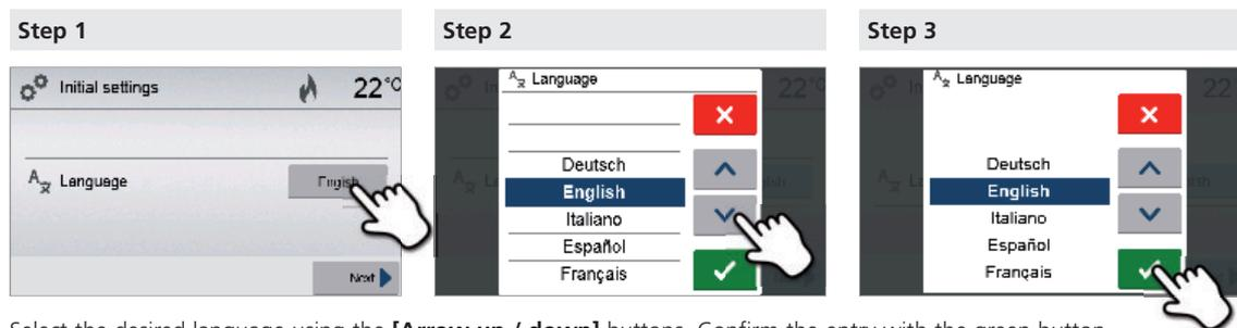
Select the desired language using the **[Arrow up / down]** buttons. Confirm the entry with the green button. The **[Next]** button is used to reach the next entry screen.
