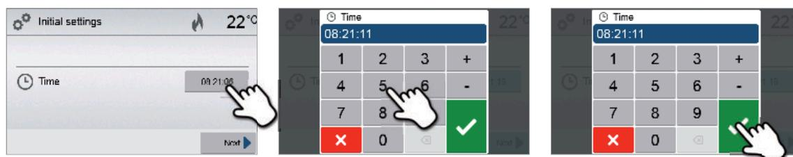
Confirm the entry with the green button. The **[Next]** button is used to reach the next entry screen.
