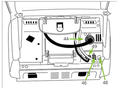
1. Insert the heater plug into the intended connector.
