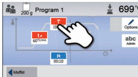
2. Enter the desired holding temperature and confirm by pressing the green button.
