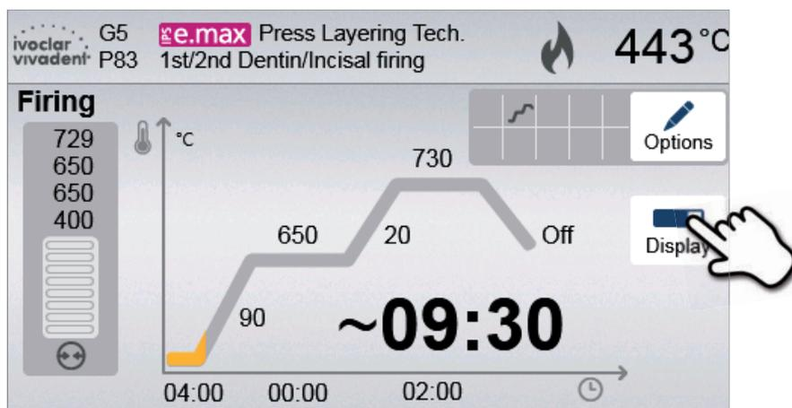
If the **[Display]** button is pressed while the firing curve is displayed, the remaining time will be shown. The remaining time indicator informs the user about the time that is left until the process is completed. The remaining time is displayed in the centre of the screen in large characters and is thus visible even from a distance.
