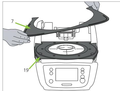
Secure the cooling tray (7) with the two screws (8).
