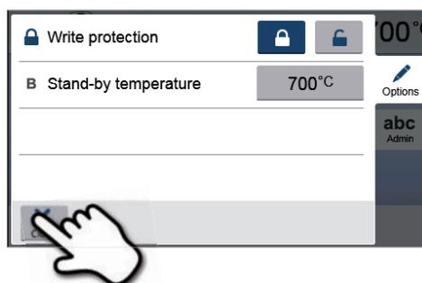
4. The write-protection was successfully activated. The lock symbol is shown next to the **[Options]** button in the display.
