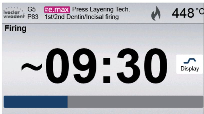
The factory settings of the furnace are such that the firing curve is automatically displayed upon the start of a program.
