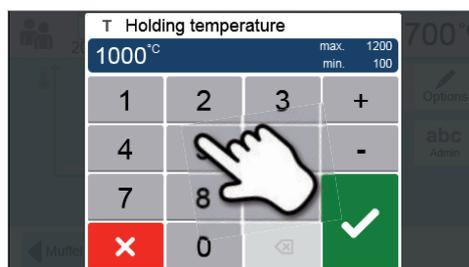
The holding temperature was successfully changed. All the other parameters shown in the firing curve can be changed / edited in the same way.
