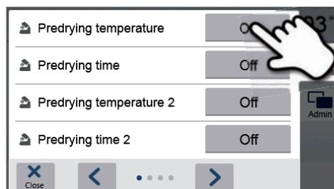
4. Enter the desired predrying temperature and confirm by pressing the green button.
