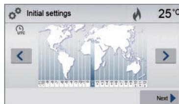
The time zone can be changed by pressing the **[Left]** and **[Right]** buttons. Use the **[Next]** button to confirm the selection and reach the next entry screen.
