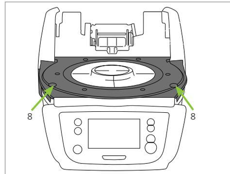
Place the cooling tray (7) on the frame plate (19). Make sure that the cooling tray is correctly positioned on the frame plate.
