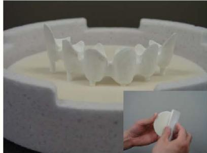
This method reduces the surface friction and allows the framework to 'slide' on flat pins as it shrinks. Make sure to frequently polish the surface of the round zirconia plate by rubbing it with a grinding stone. This plate is from Katana, Noritake and works well to prevent "deformation" of your framework. (for DelCam and other open CAM software users)
