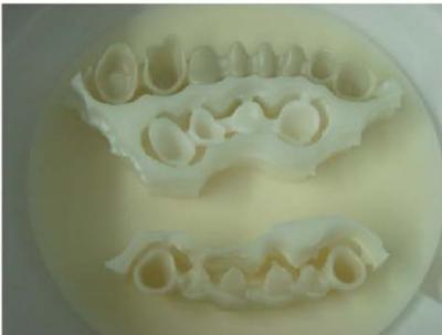
This proven method employed by experienced technicians is especially effective for large unit bridges. The "holding" effect of the extra support of zirconia prevents the warping of large unit bridges with dense pontic areas that shrink comparatively more than the abutments
