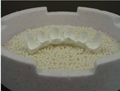
Ensure that the entire surface of the substructure is supported by the sintering beads. This avoids deformation. Care should be taken to prevent sintering spheres becoming "jammed" in the connector areas. (for Sirona Cerec, MC-XL users)
