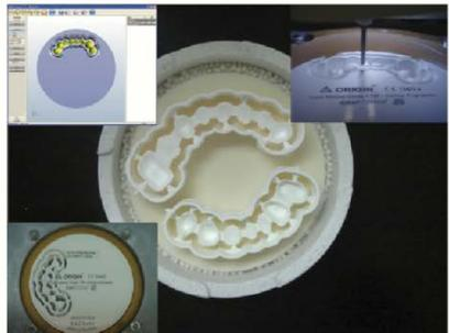
This is another proven method for medium to large unit bridges used by outsourcing centers. The surrounding wall automatically designed by CAM software provides for uniform and even shrinkage. It prevents deformation even though there are dense pontic areas that shrink substantially more than the abutment copings. (ORIGIN CAM software users)
