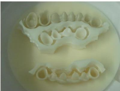
This proven method employed by experienced technicians is especially effective for large unit bridges. The "holding" effect of the extra support of zirconia prevents the warping of large unit bridges with dense pontic areas that shrink comparatively more than the abutments
