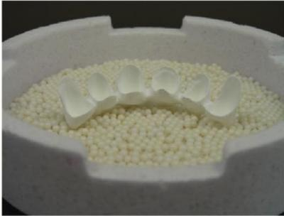
Ensure that the entire surface of the substructure is supported by the sintering beads. This avoids deformation. Care should be taken to prevent sintering spheres becoming "jammed" in the connector areas. (for Sirona Cerec, MC-XL users)
