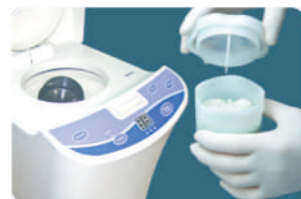
3. Close tightly the cap of mixing bowl
