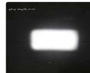
The beam spot is rectangular and the size is moderate. (80x160mm at 700mm) And no dazzle light around
