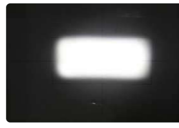
The beam spot is rectangular and the size is moderate. (80x160mm at 700mm) And no dazzle light around
