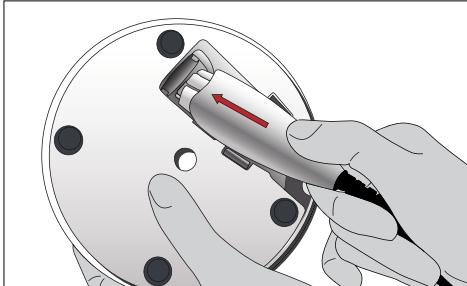
Connect the power cord with the power supply and the power pack. The Power On indicator on the power pack lights up in green and the illuminated ring on the charging base briefly lights up.
