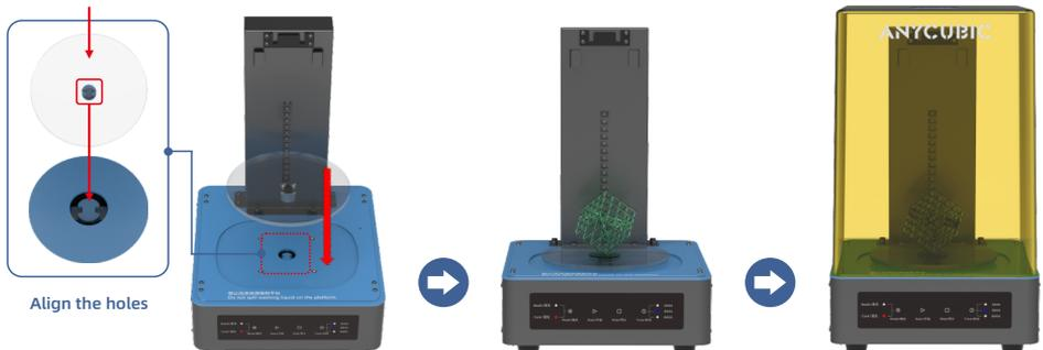
3. Select the curing time. (Generally, if a model has a diameter of less than 30mm, it is recommended to have a curing time of 2 minutes. If the model has a very complicated surface structure, it is recommended to increase the curing time.) Then touch the start icon to start curing the model.
