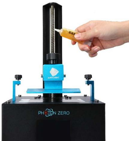
(1) If Z axis make noisy sound, please apply lubricant to Z lead screw.
