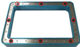
(5)The FEP film may lose the tension over time and usage. Please adjust the tension by tightening the screws at the bottom of the resin vat.
