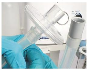
6. Attach the filling tube (1700 mm) on one end with the angled connector (optional REF 28535) and the other end of the tube with the instrument.
