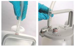
8. Graft the angled connector (optional REF 28535) of the filling tube (1700 mm) onto the wider nozle (PA-TIENT) of the secretion jar. Hang the other end of the filling tube with the instrument into the quiver.
