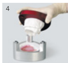
4 After the setting time of the plaster open the POLYMASTER. Let the mixed AESTHETIC BLUE flow into the counter, the gingivo-buccal fold and palate of the model.
